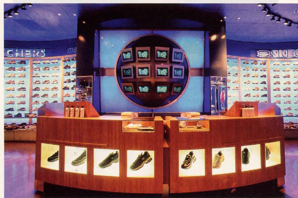
Within the cashwrap counter's face are eight internally lit, hollow, glass boxes showcasing a specific shoe style. These floating shoe displays mimic the omnipresent monitors above.
